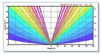
**Figure 5** – NEXRAD beam heights with distance for various antenna elevation angles in precipitation mode.
