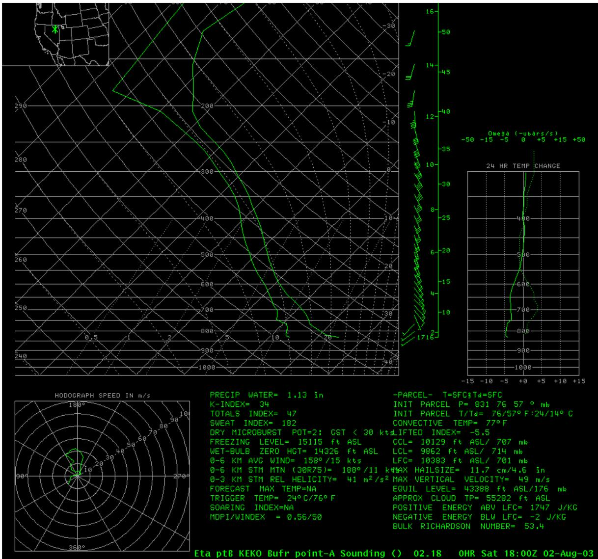
Fig. 3. 1800 UTC Eta Bufr sounding showing continuing trend toward moist and unstable environmental profile with relatively weak shear.
