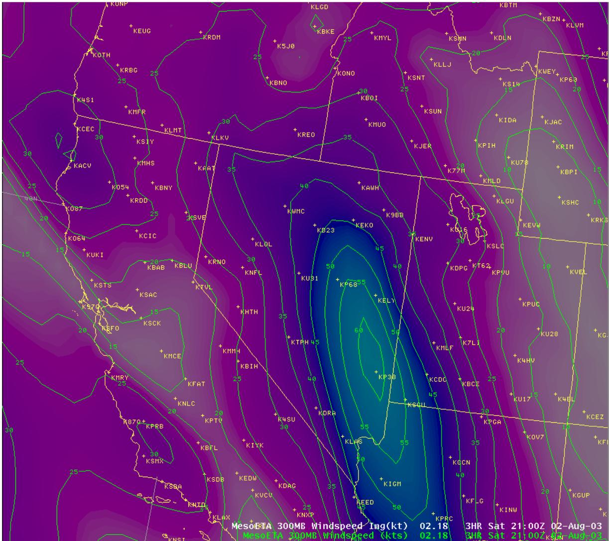
Fig. 6. 2100 UTC ETA40 (MesoEta) forecast of 300mb jet max moving from Central Nevada into Elko County during thunderstorm development.
