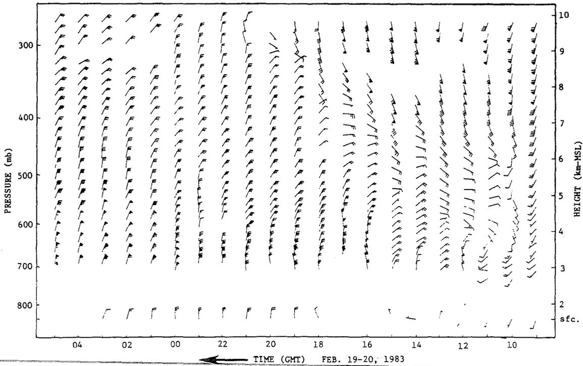
FIGURE 4. - This graphic represents a 24-hour history of 1-hour profile averages for one profiler site in northeastern Colorado. Note the passage of a low level disturbance between 10-12Z and its reflection in the upper levels at later times.
