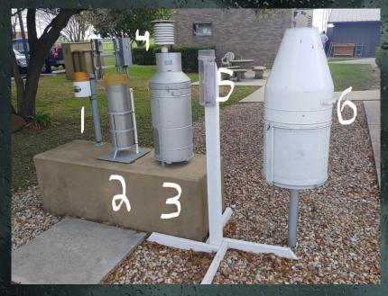
Gage #1 is a "Tipping Bucket" gage, and it's our most commonly used *near-real time automated* rainfall measurement device. The gold top portion is a funnel that drips down into a little triangular "bucket" that tips over and empties once it's reached a set amount. After tipping, a second "bucket" faces up, which repeats the process and tips back when full (see the schematic below.)
